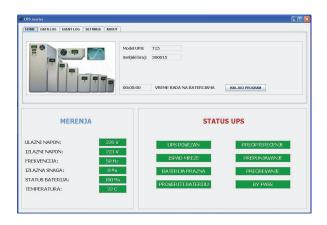
• An option of installing a LAN card with SNMP and HTTP protocols, which allows real-time monitoring of UPS devices anywhere in the country and abroad.
